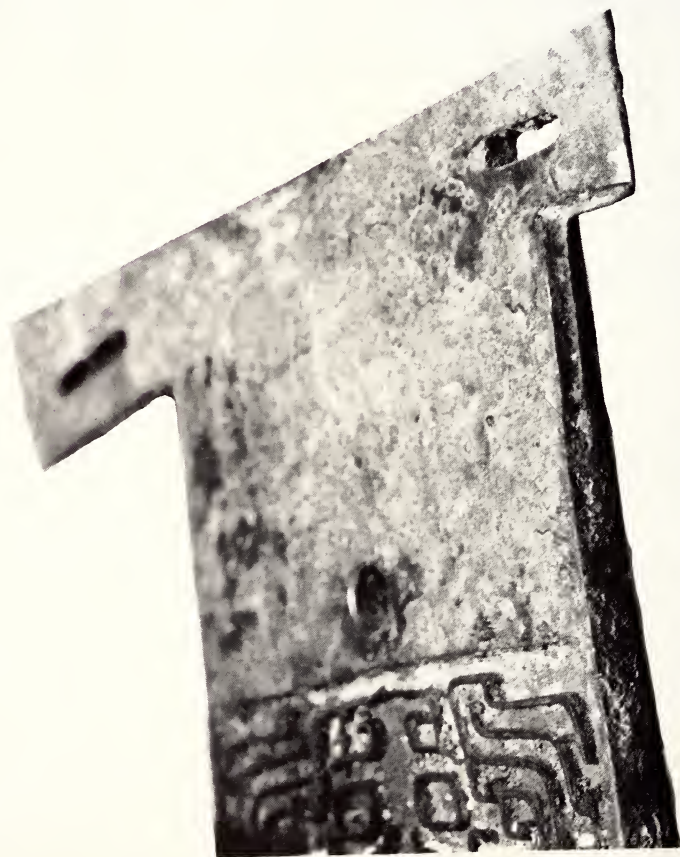
FIG. 3.—34.10. Chinese bronze broad axe of the type ch'i with iron blade. Detail ( \times 1.7 ) showing a ridge along edge of the tang which is the flash (mold mark) left at the juncture of the two halves of the mold in which the axe was cast.
